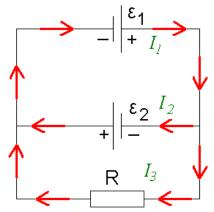
And as shown above, the following notation flowing currents. Let the two battery packs and the currents flow  $I_1$  and  $I_2$  respectively, and the current flows through the resistor  $I_3$ .
